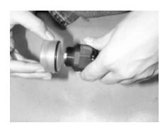
7. Screw the lens over the end of the fiber tight connector until the o-ring makes a tight seal.
