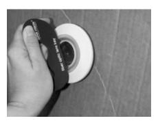
10. Tighten the retaining ring snug.
