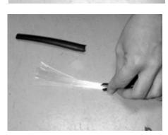
2. Inspect the fiber for any damage. Re-cut if necessary.
