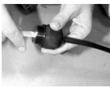
4. Tigten the fiber-tight connector over the black jacket. Check that the fiber will not pull out.
