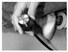
6. A smooth cut should result. If the cut is not smooth, loosen the fiber-tight connector and push the fiber through so another cut can be made. Make sure the fiber-tight connector is tight before cutting.
