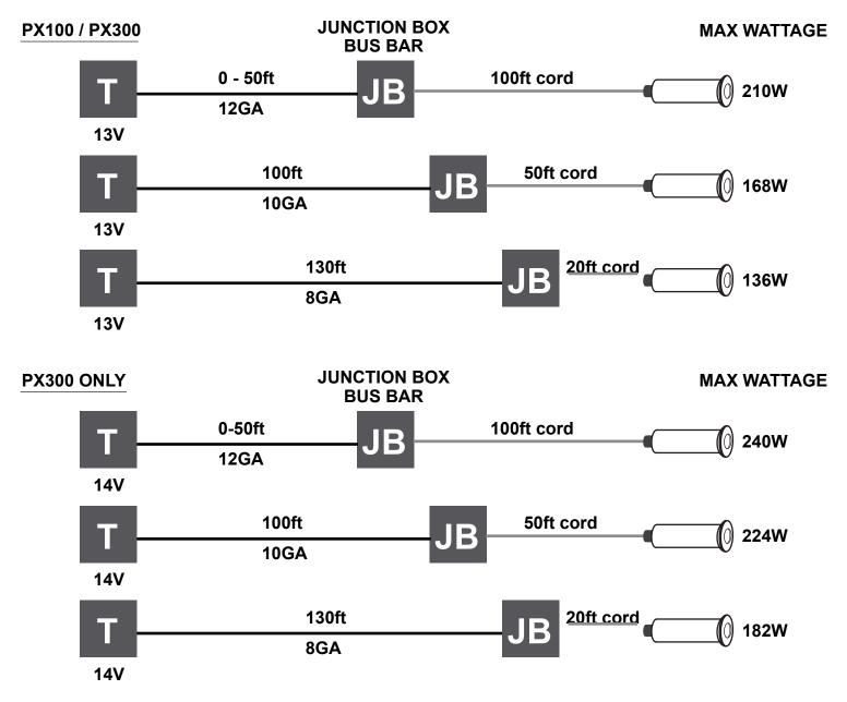
NOTE: Please use appropriate low voltage supply to pool lights, ie. if 12V is appropriate voltage DO NOT use 13V or 14V tap on transformer output (if so equipped),
