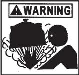
**This filter operates under pressure. If this unit is not assembled properly or is operated with air in the circulation system, serious bodily injury and/or property damage could occur.**
