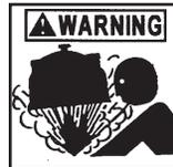
**If filter Ring-Lok is not tightened to “built-in stops”, filter lid could blow off causing injury or property damage.**
