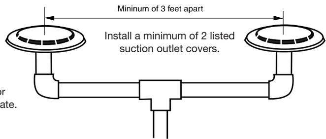
Each main drain shall be rated at or above the maximum system flow rate.
