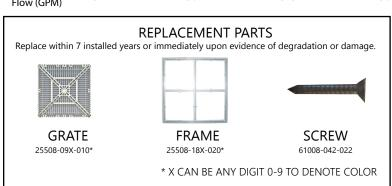
**WARNING:** To reduce the risk of drowning from hair and body entrapment, install suction fittings with a marked flow rate in gallons per minute that exceeds the flow rate of your system by at least 25%. Always use multiple suction outlets. If the fitting/cover breaks, is damaged, or is missing, shut the system down immediately. Do not use the system until damaged parts have been replaced.
