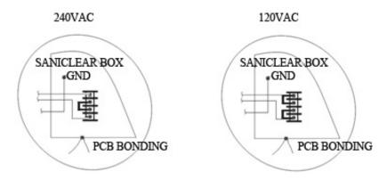
At the bottom of the Salt chlorinator there is a connection that should be used to ground the unit to the pool grounding system with a copper wire of 8 AWG (6 AWG for Canada) (as per diagram below)
